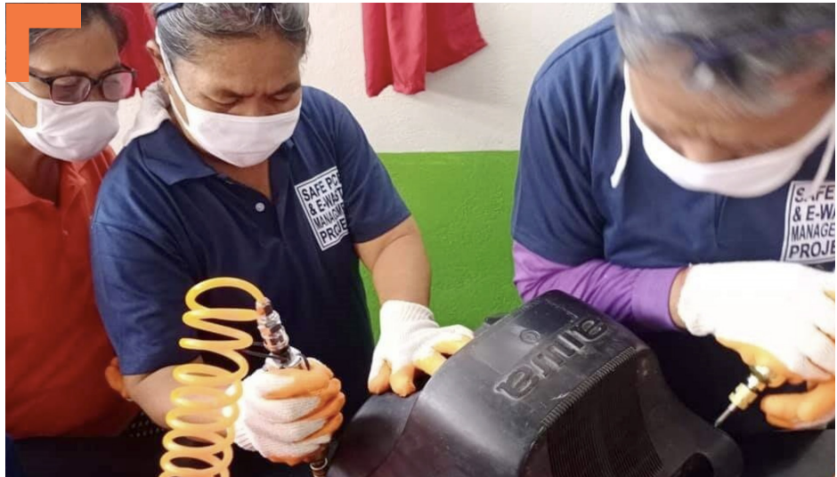
Women wearing personal protective equipment using pneumatic tools to dismantle electronic devices
